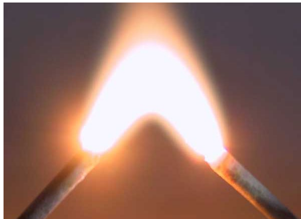
Figure 1: An electric arc generated using two electrodes. Image courtesy of Achim Grochowski–Achgro, own work, CC BY-SA 3.0
