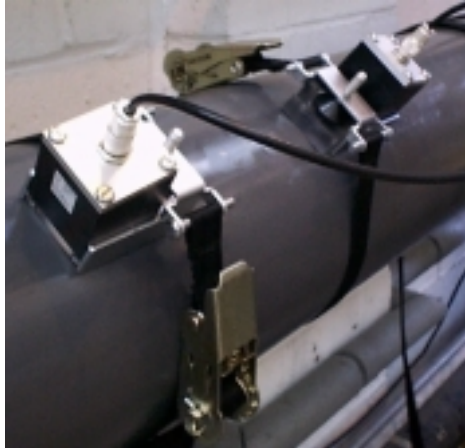
Figure 11 – Reflex Mounting for Transducer Set 'D'
