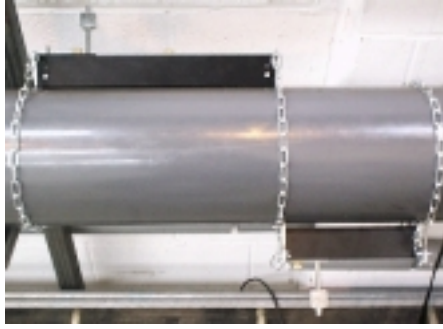
Figure 11 – Reflex Mounting for Transducer Set 'D'
