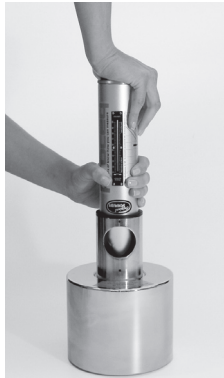
Fig. 3.1 Performance check of the concrete test hammer (model N/L shown)
