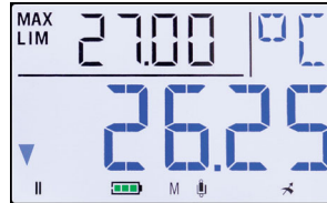
1. Measured value (blue) below the limit 2. Limit
