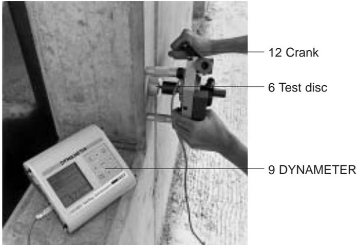
Fig. 5.6 Measuring procedure
