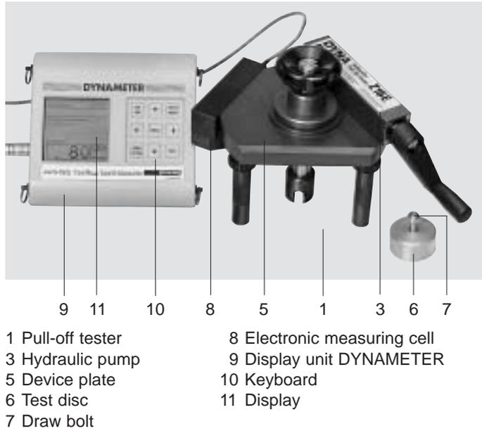
Fig. 2.2 DYNA Z...E Pull-off tester, with display unit, DYNAMETER
