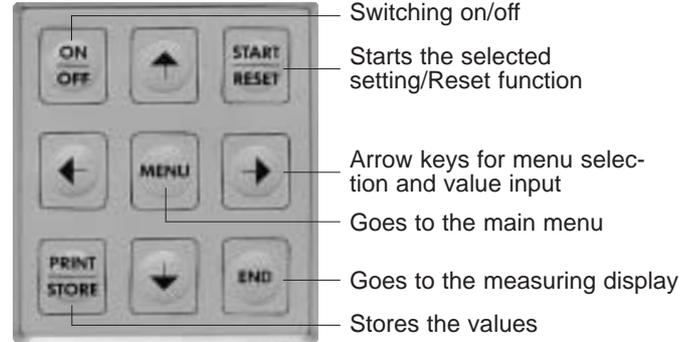
Fig. 3.4 Keyboard (10) of the DYNAMETER
