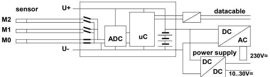
The analog inputs are electrically isolated by means of photo voltaic relays; the maximum potential difference permitted between them is 50 VDC or 60 VAC. Sensors combined within one connector and sensors with their own power supply, however, are electrically interconnected and must therefore be operated in isolation. The voltage at the measuring inputs themselves must not exceed 5 volts (between B, C, D, A and -).
