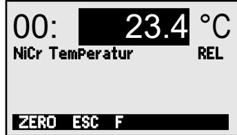
To select the **zero-set measured value function** press **<ZERO>**.
