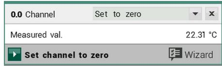
confirm via selection box '**Zero-set**'. The measured value is then saved as **base value** and thus set to zero. To save the relative reference value to RAM on a temporary basis only, option 'Temp. zero-setting' must be used. (**Display 'REL'**)
