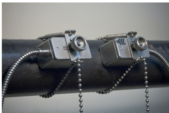
Illustration 7: Sensor mounting with clips and chains
