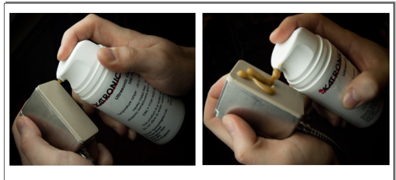
Illustration 5: Application of acoustic coupling gel
