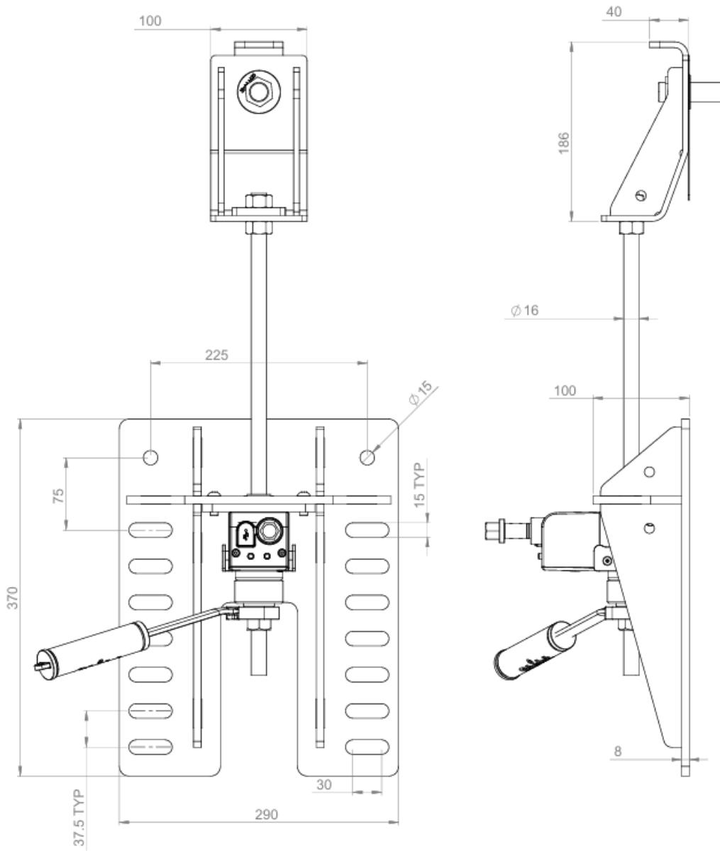
**Application** – For shear testing fixings from M6 to M20 to MAX 60kN. Can be used with a t25 or t60 load cell.
